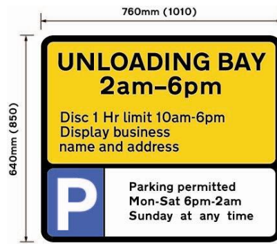
Plate indicating alternate use, and times and conditions of use as unloading bay (above) and parking place (below) 640.1J
