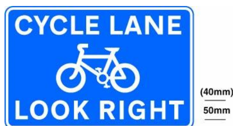
Cycle lane with traffic proceeding from right (Sign for pedestrians) Permitted variants: "RIGHT" may be varied to "LEFT" or "BOTH WAYS". "LANE" may be varied to "LANES" or "TRACK". The symbol may be reversed. 963.1
