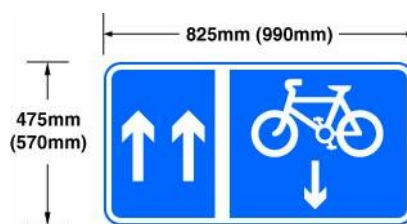
Contra-flow cycle lane Permitted variants: route symbols or the number of arrows or symbols indicating which lanes are open or closed may be varied Use with diagrams 1049 and 1057 960.1
