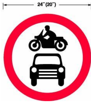
All motor vehicles prohibited (See Article 7) 619
