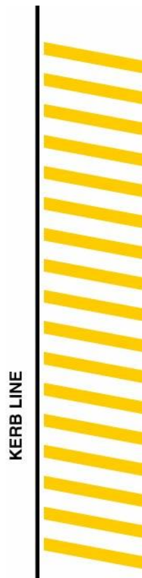
Marking to be placed on the side of a road to indicate that stopping by vehicular traffic on that side is prohibited along the length of the marking (See Articles 14 and 17) 1016J
